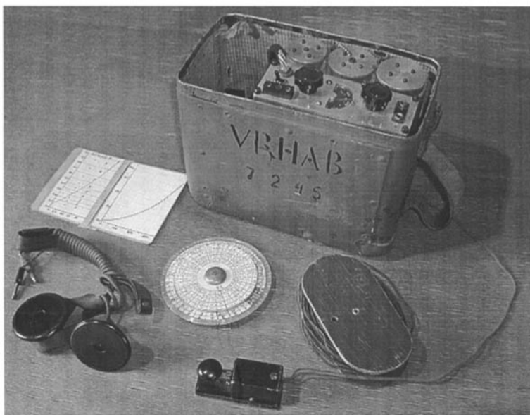
Kyynel transmitter M 4 and receiver M 7 combination (also known as 'VRHAB') with accessories packed in a cardboard transport case having a leather-effect paper covering and reinforced corners. Note antenna reel, cipher dial (round object in centre) antenna length setting chart and calibration charts for receiver and transmitter tuning dials
