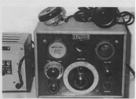
Mk.V fitted in wooden box (above left). Note plug-in coil units for different frequency ranges. Mk.V receiver, probably a stand-alone variation with associated AC power pack (above right)
