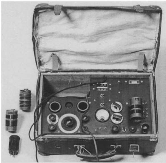
Mk.V suitcase variation, receiver section on the left and transmitter with built-in AC mains power unit right
