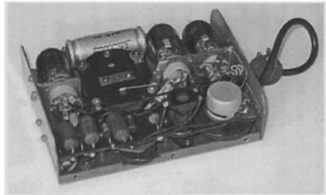
Internal view of Midget Receiver Type 53/I showing the three type 9001 valves, tuning capacitor and its associated reduction gear (centre), tuning coil and reaction control potentiometer (right)
